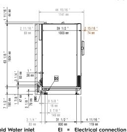
CWI1 = Cold Water inlet CWI2 = Cold Water Inlet 2
